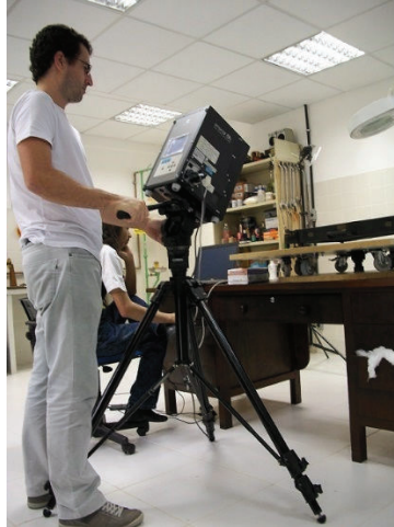
FIG. 3 - The Konica-Minolta scanner during a digitization session of the Bamberg's lower base.
