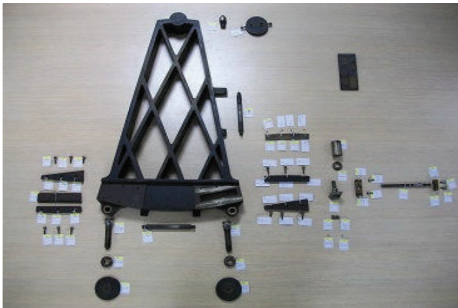
FIG. 2 - The Bamberg's lower base completely disassembled. Each part is labelled and kept in its respective place to guarantee the correct assembly afterward.
