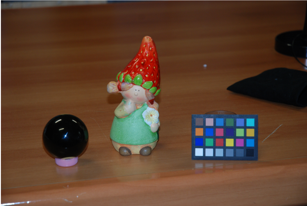
Figure 4.3: Our typical acquisition environment consisting of the target object, a reflecting sphere to extract light direction, and a color chart for calibration purposes.
