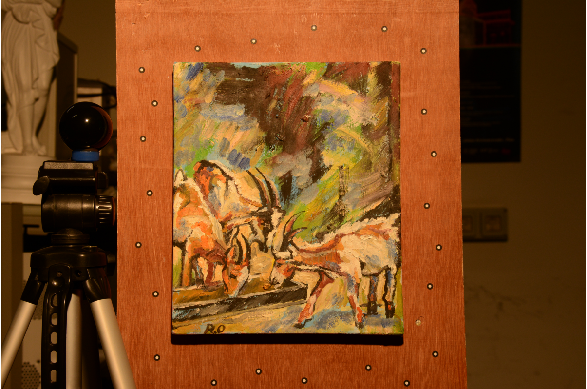
Figure 4.4: Demonstration of a sphere used to capture the light direction
